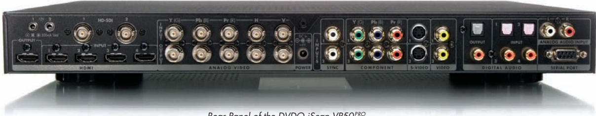
Rear Panel of the DVDO iScan VP50 PRO
